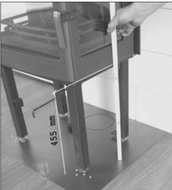
Fig 8 Locate the hearth unit on the metal plate in accordance with the markings (Fig. 4). Adjust the height to approximately 455 mm, measured from the floor to the lower edge of the cast-iron sidepiece. The flue centre must be 150 mm from the wall.
