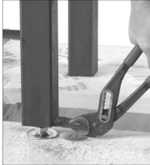
Fig 7 Remove the transport attachment from the front leg. Use a polygrip tool, or cut it off with a metal saw.
