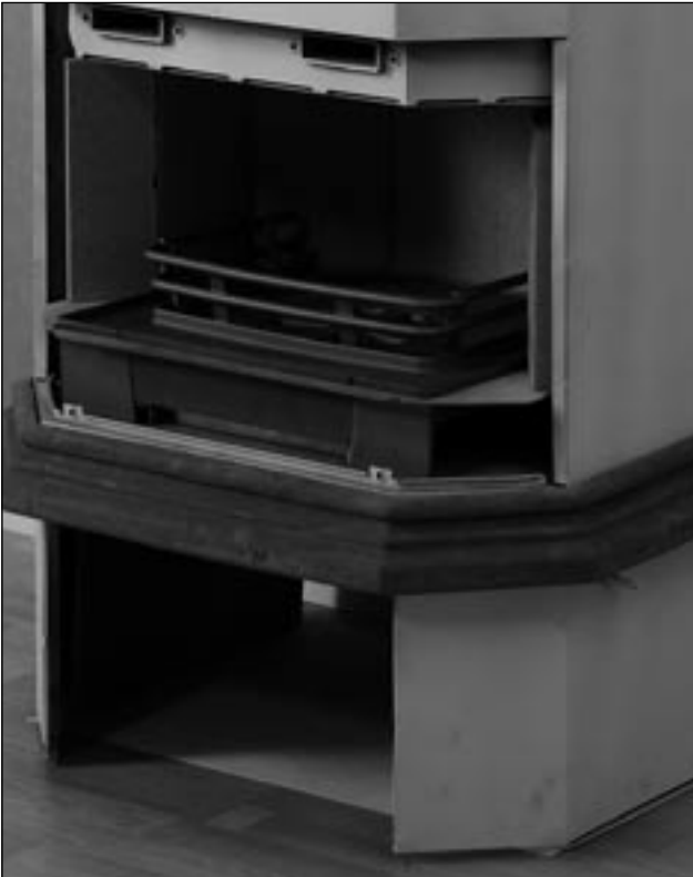
17. Screw the foot-moulding support brackets in place and apply silicon to attach the moulding. Make sure the height is correct, otherwise it will be impossible to fit the door front. You should also check that the foot-moulding is horizontal. N.B. The support brackets are only used during assembly, and should be removed after the adhesive has dried, prior to painting.
